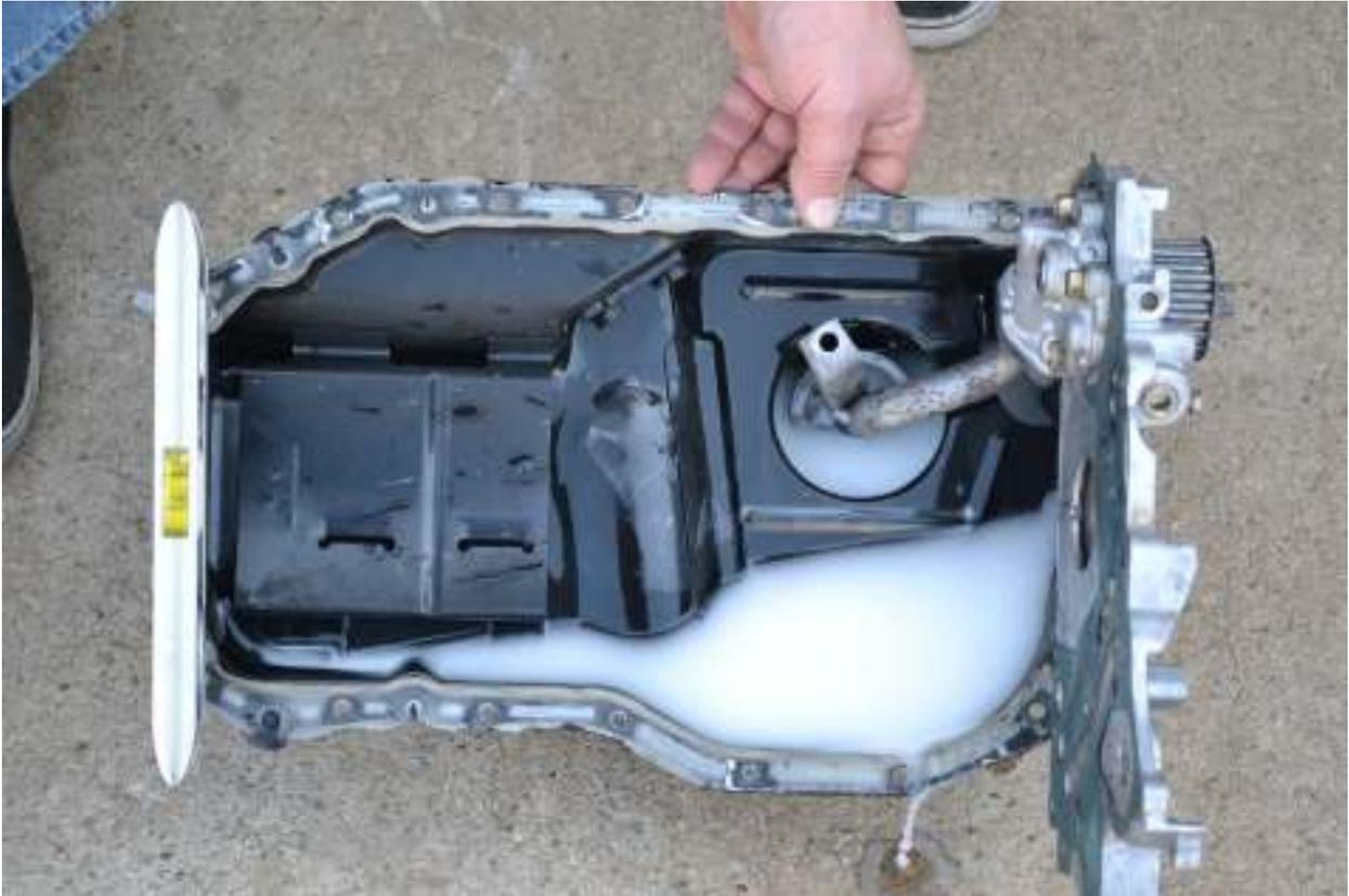
The next question is how do you fix it? Well from our point of view it's put a ball bearing turbocharger on the car. Ball bearing turbochargers can live with intermittent oil supply without any damage. From the complete systems perspective the answer isn't so obvious. Baffle the oil pan, relocate the oil pickup towards the middle/back of the pan, install a dry sump, or operate at 275hp so that the oil system can operate as it was designed , but that's no fun.
